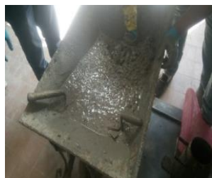
Fig (4): Fresh geopolymer concrete
