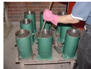
Fig (7): Compacting geopolymer
